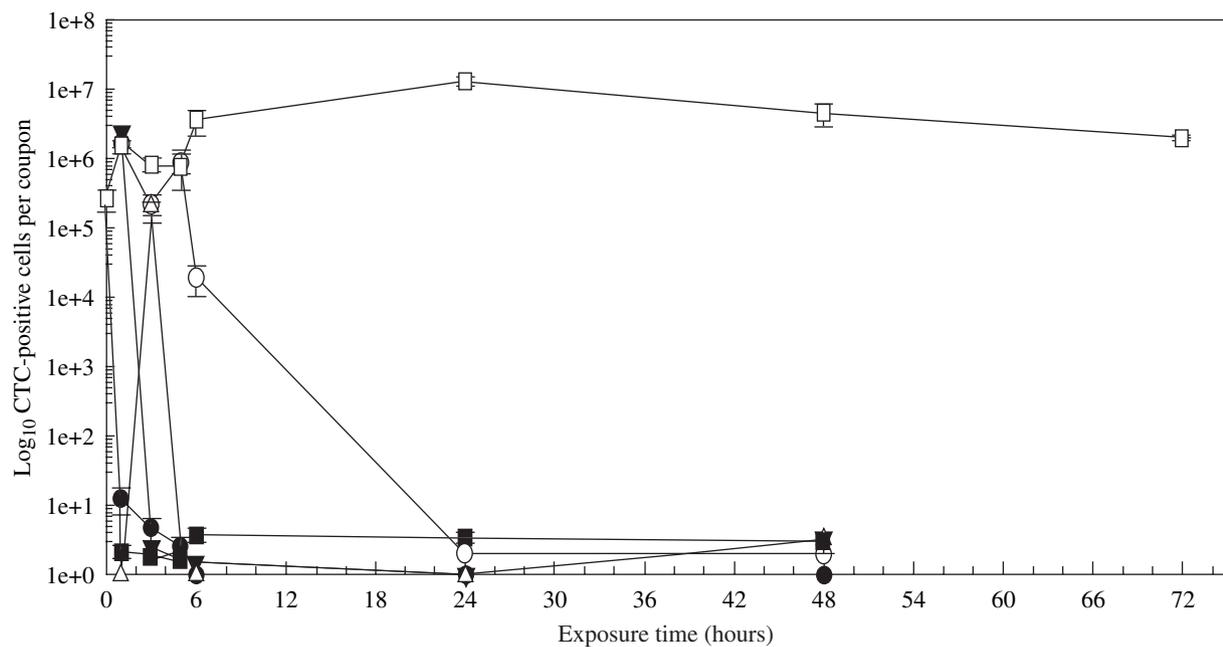
**Figure 4** Effect of *C. difficile* (spores) viability after exposure to C11000 (●), C26000 (○), C51000 (▼), C70600 (△), C75200 (■) or S30400 (□) at 22 °C, using SYTO9 and CTC staining. Data points represent mean (N=6) ± SEM.
