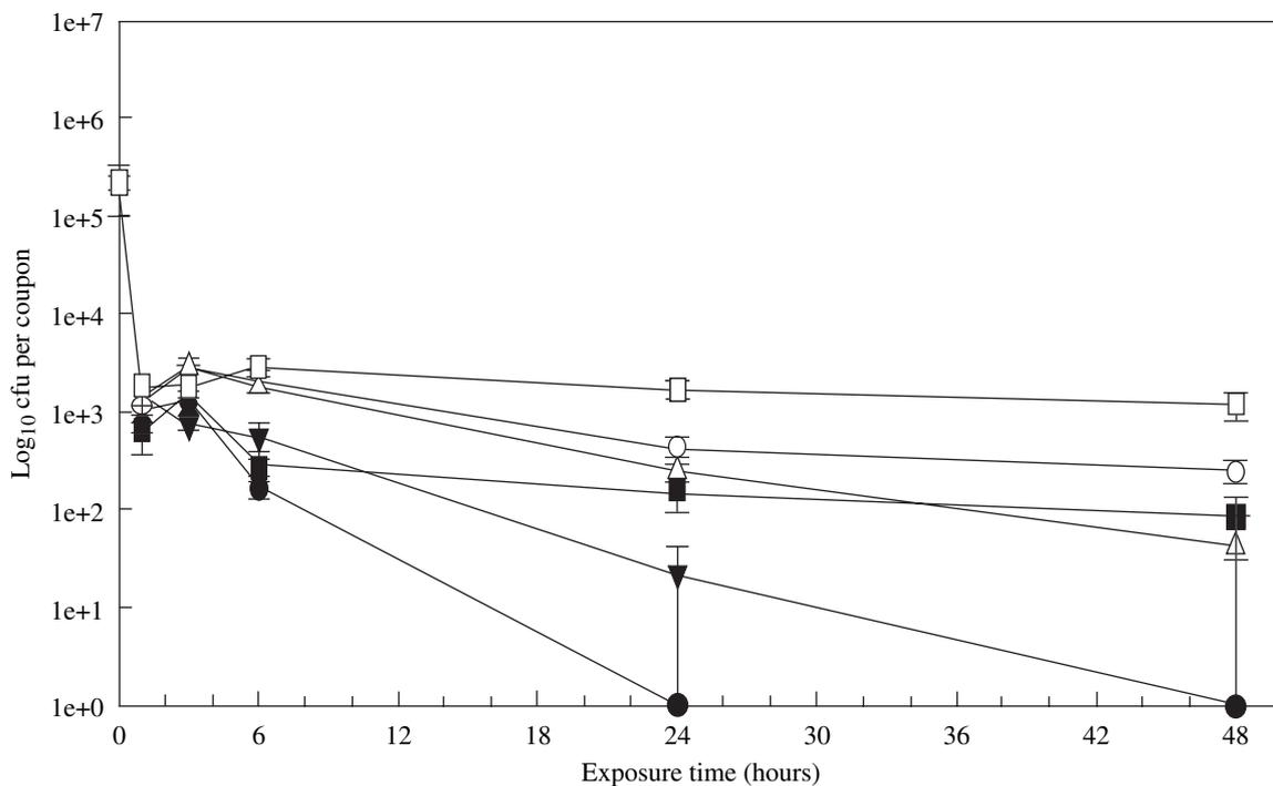
**Figure 2** Effect of *C. difficile* (purified spores) viability after exposure to C11000 (●), C26000 (○), C51000 (▼), C70600 (△), C75200 (■) or S30400 (□) at 22 °C, using SYTO9 and CTC staining. Data points represent mean ( $N = 6$ )  $\pm$  SEM.
