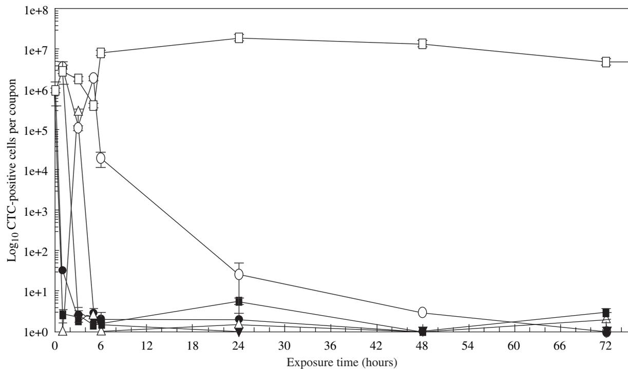
**Figure 3** Effect of *C. difficile* (total vegetative cells and spores) viability after exposure to C11000 (●), C26000 (○), C51000 (▼), C70600 (△), C75200 (■) or S30400 (□) at 22 °C, using SYTO9 and CTC staining. Data points represent mean (N=6) ± SEM.
