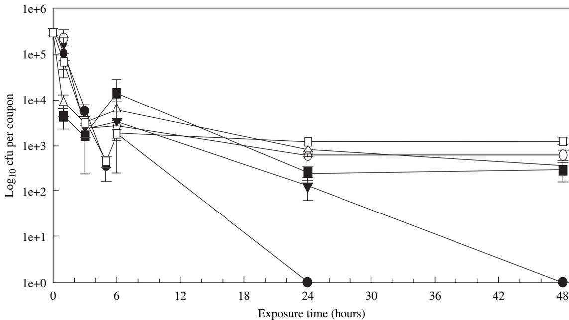
**Figure 1** Effect of *C. difficile* (total vegetative cells and spores) viability after exposure to C11000 (●), C26000 (○), C51000 (▼), C70600 (△), C75200 (■) or S30400 (□) at 22 °C, using plate count method. Data points represent mean ( $N = 6$ )  $\pm$  SEM.
